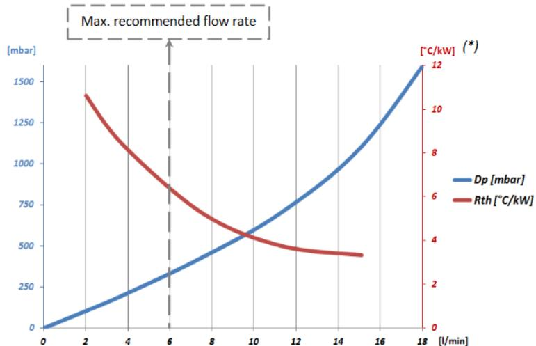
(\* )  $R_{th}$  :LCP surface to inlet water by homogeneous power loss distribution (Water + Ethylene Glycol 50%vol. @40°C)
